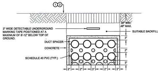
**1 CONCRETE ENCASED DUCTBANK
