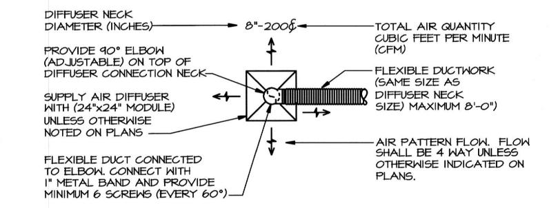
SUPPLY AIR DIFFUSER KEY NO SCALE
