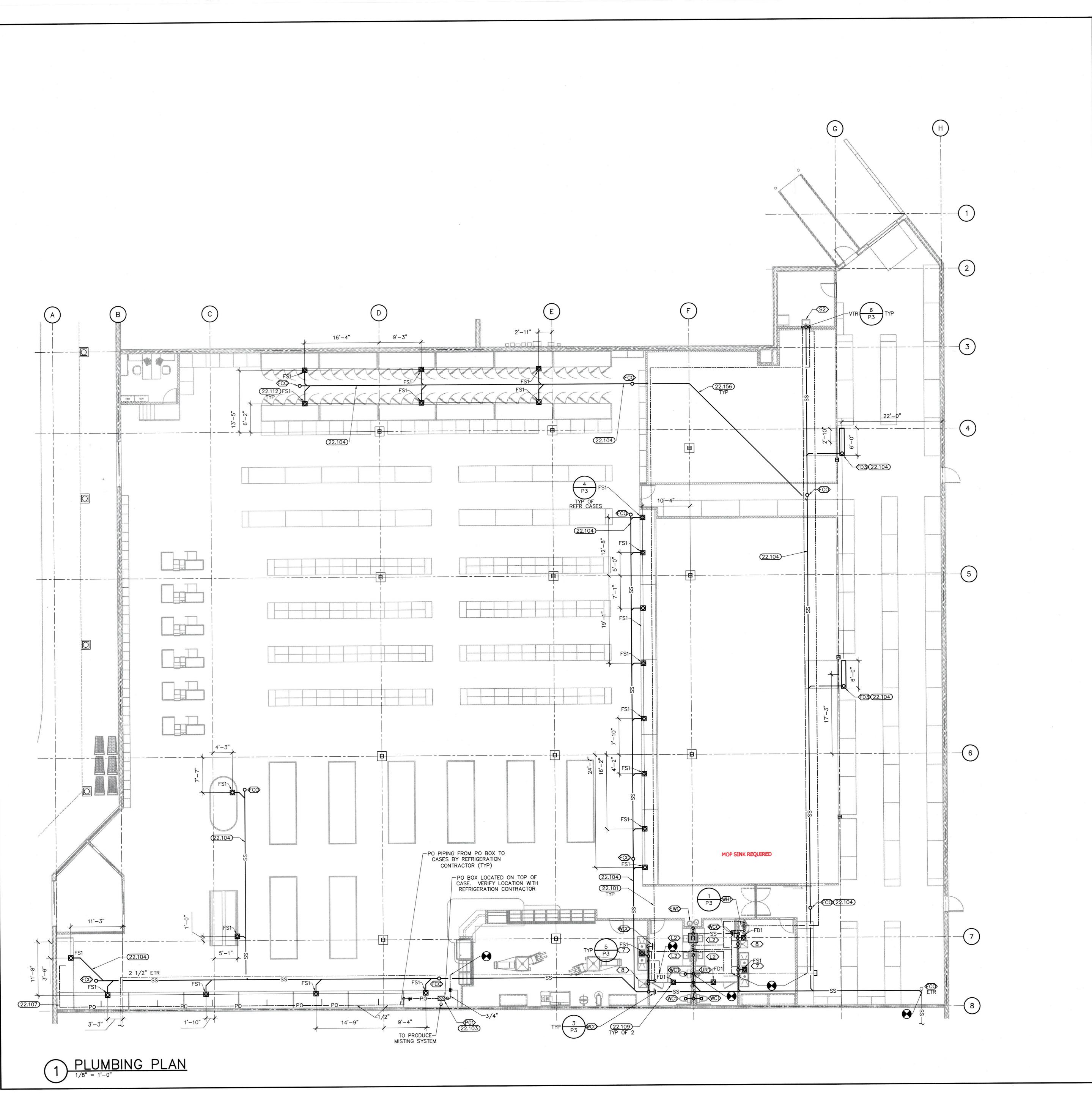
22.101 ROUTE PIPING THROUGH JOIST SPACE. COORDINATE WITH HVAC, FIRE PROTECTION AND OTHER TRADES.
